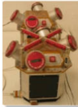
Figure 11-2: Busek colloid clusters delivered to JPL for the LPF mission (Credit: Busek)
