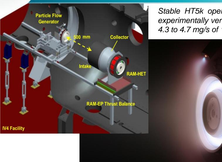
Stable HT5k operation with atmospheric propellant was experimentally verified at 225 V and at AMFR ranging from 4.3 to 4.7 mg/s of  $1.27N_2+O_2$  mixture.
