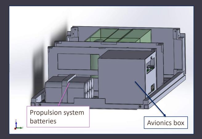
Propulsion system batteries are Li Ion battery packs 14,8 V and max current 5.2 A. They are strictly dedicated to provide electrical power supply to Propulsion System.
