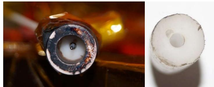
Breadboard model after  $\sim 2000$  pulses
